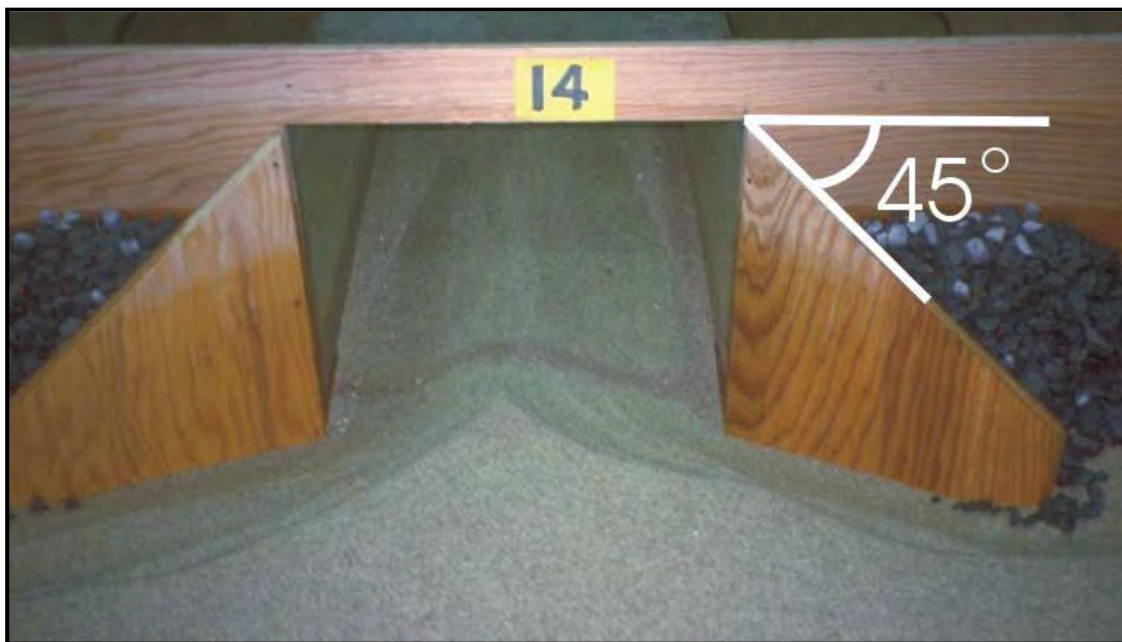
Figure 6.16. Rectangular model with wing walls (FHWA 2003a).
