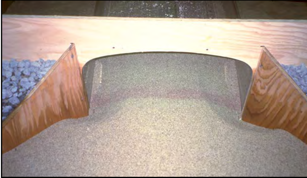
Figure 6.17. Arched model with wing walls (FHWA 2003a).
